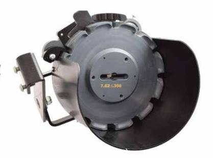
The bullet feeder shown here is being prepared to mount to a 650 (with the case feeder to the left of the bullet feeder).
