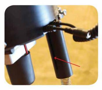
The spring adaptor cap fits on top of the switch section in the dropper assembly, with its flat side facing the switch. There is a set screw in the side of the part – screw that in to hold it in place. The screw will enter into a groove in the switch section. Again, do not over tighten!
