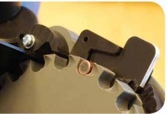
In the left image, not enough spacers are used in the nose guide for this 124 gr 9 mm bullet, and consequently the bullet's base is dropping too low below the level of the top of the collator plate. In the right image, extra spacers have been added into the nose guide  $(2 \times 1.6 \text{ mm})$  and  $(2 \times 1.6 \text{ mm})$  and the bullet is now entering to the correct depth.
