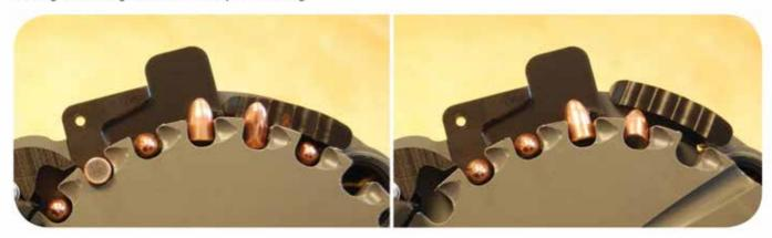
The left image shows the correct ramp position for these 9 mm bullets – the ramp is close up against the collator plate and so the bullets can ride up the ramp and complete their rotation. In the right image, the ramp is positioned much too far out for these bullets, and the bullet tip is missing the ramp and jamming up beneath it.
