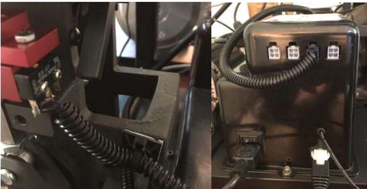
Figure 29: Cable assembly with strain relief, Port to plug into console.
