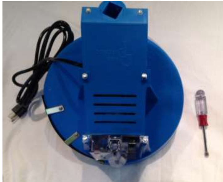
Figure 56: Case Feeder cover ready for removal
