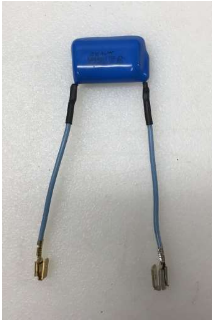
Figure 16: Case Feeder RC Filter
