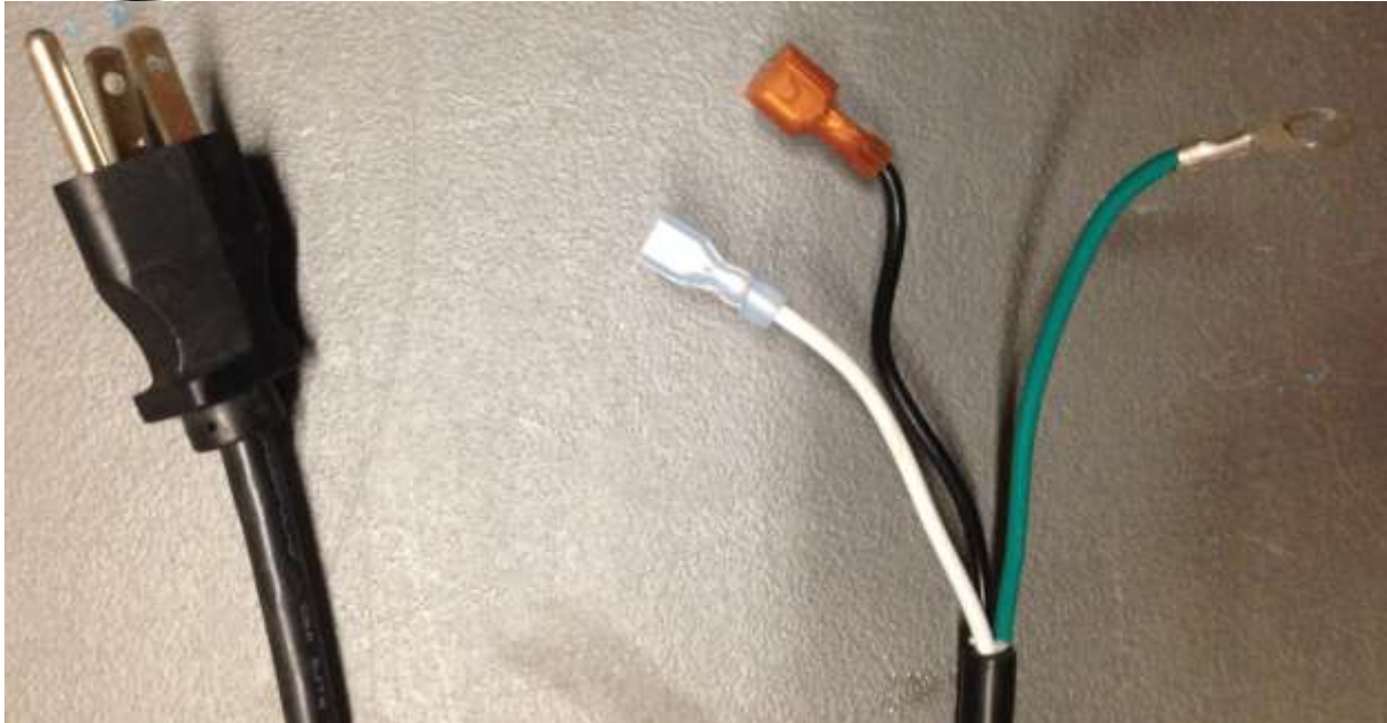
Figure 59: AC Power Cord with Female Spade terminal installed
