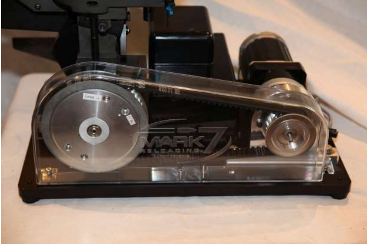
Figure 6: Belt Guard Installed
