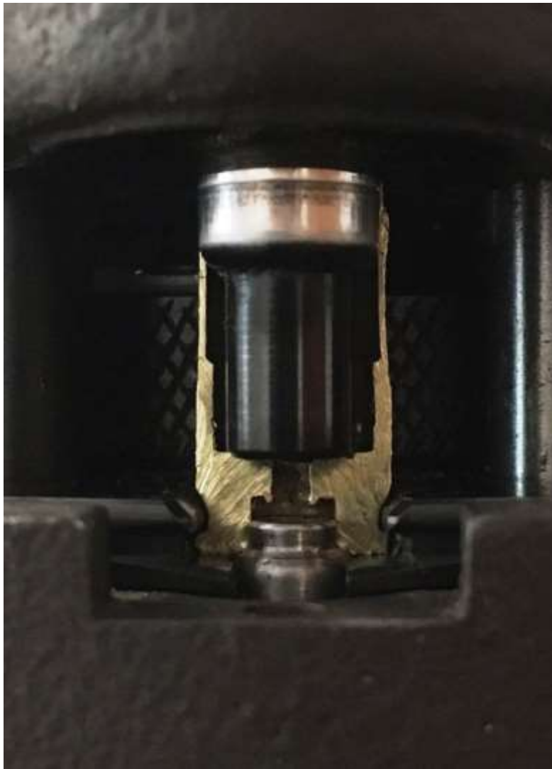
Figure 30: Cross-section of properly adjusted Swage Rod
