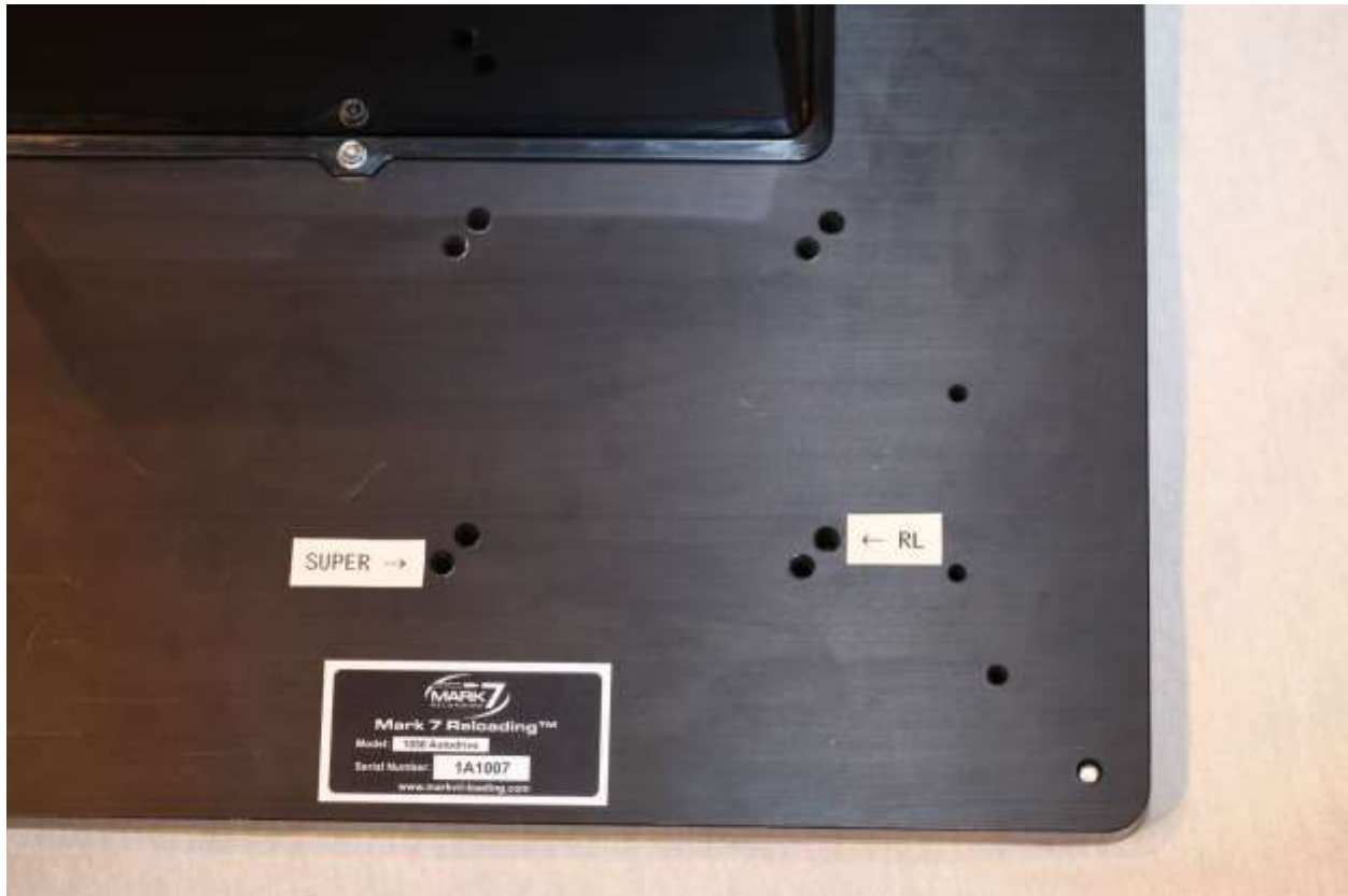
Figure 2: Mounting Location on baseplate for RL and Super
