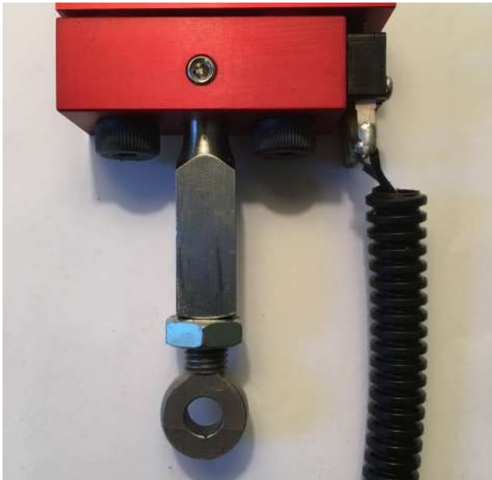
Figure 27: Rod end installed
