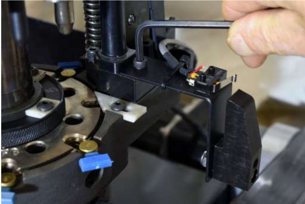
Figure 36: Installing the Shield Latch
