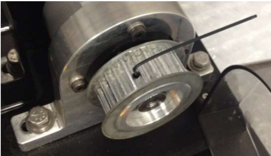
Figure 49: Adjusting the small sprocket position on the gearbox shaft
