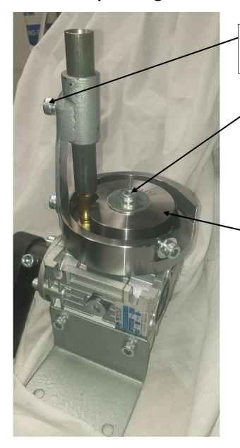
Socket head bolt to adjust drop hose height and to allow calibre conversions to be changed.
