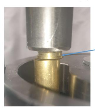
The full extractor groove of the case above must be visible
