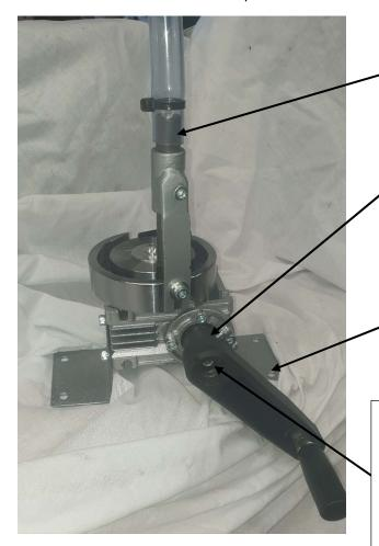
Drop hose showing PVC hose correctly positioned. Trim the **other** end if you need to shorten the hose.
