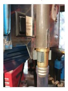
The brass adaptor will clip into the casefeeder where the normal plastic drop hose connects the Dillon™ casefeeder to the Dillon™ reloading press. The flexible PVC hose supplied will connect the brass adaptor clip to your rollsizer drop hose.
