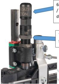
6A. Remove this cap to remove / replace the Guide Rod / decapping pin
