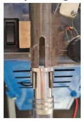
The adaptor will clip into the casefeeder where the normal plastic drop tube connects the Dillon™ casefeeder to the Dillon™ reloading press. The flexible Vinyl hose supplied will connect the adaptor clip to your Decapper drop tube.
