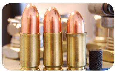
The resulting bullet seating of the three powder funnel heights. The left bullet is not seated well, as the funnel is too high – and as a result the bullet is likely to tip over as you index the machine. The middle bullet is well tapped into place, and will remain straight and true as you index. The right bullet shows the result of belling the case too much. The deformation in the case will cause rapid case fatigue, and the bullet may not remain straight as you seat it.
