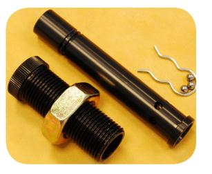
To reassemble, slide the inner tube into the threaded body from below until the row of holes is just visible. Position the three steel balls on the same level of holes (each separated by 120 degrees) and slide it further up until the threaded body retains the balls. Then slip the retention spring back into place. Use the upper groove when using the upper row of steel-ball pockets (normal setup) and the lower groove when the steel balls are positioned lower for very short bullets.
