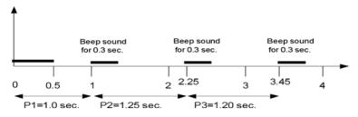
(The above example shows three Par times being activated by a single start beep. A total of four beeps will be emitted from the timer. One START beep and three PAR beeps at the intervals selected. Each PAR time entered will be based from the previous one. Therefore in the above example, from the timer activation (start beep), the next beep will begin at 1.0 second, followed by another beep starting at 2.25 seconds, with the final beep starting at 3.45 seconds.)
