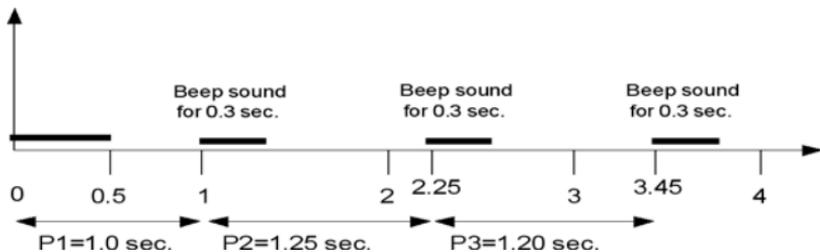
(The above example shows three Par times being activated by a single start beep. A total of four beeps will be emitted from the timer. One START beep and three PAR beeps at the intervals selected. Each PAR time entered will be based from the previous one. Therefore in the above example, from the timer activation (start beep), the next beep will begin at 1.0 second, followed by another beep starting at 2.25 seconds, with the final beep starting at 3.45 seconds.)
