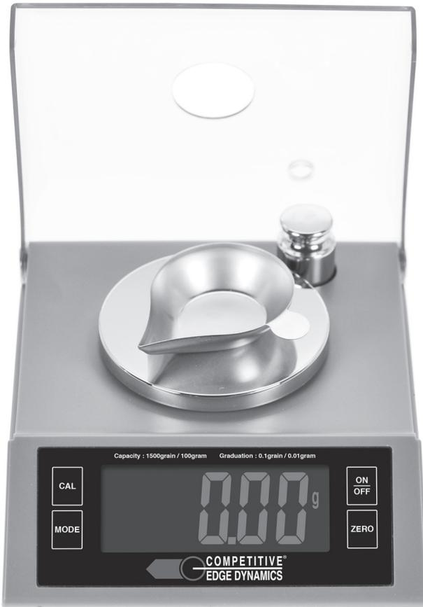
4. Press the ZERO key to "zero out" the scale. This will remove the powder pan weight allowing only the powder itself to be weighed. This function is called "TARE Function" *FIG 11*
