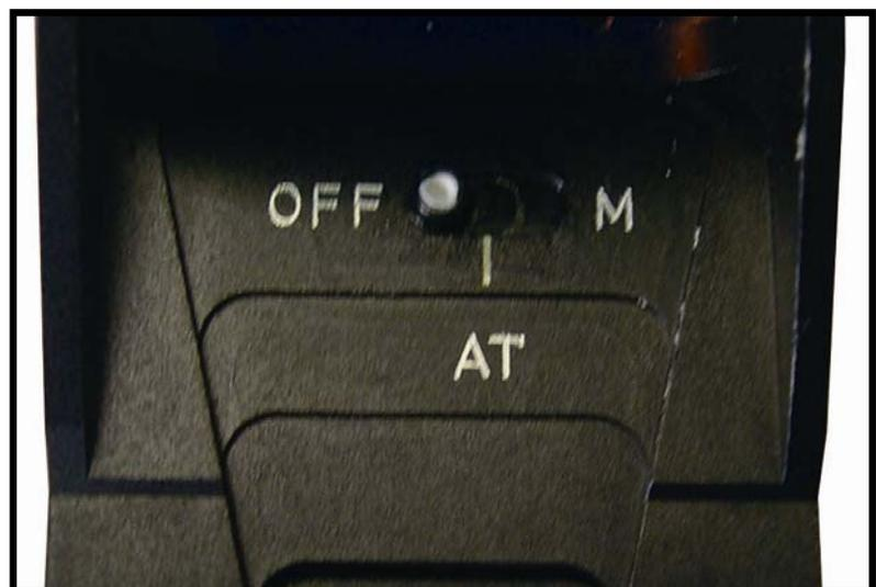
manual override marked M which will provide a brighter setting than available with the use of the Photo sensor. Please ensure you return the switch to the OFF position after use to avoid battery failure. Note replacing the cover does not turn the sight off.
