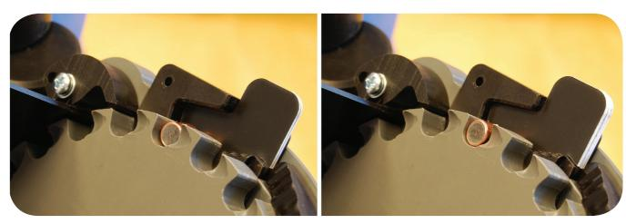
In the left image, not enough spacers are used in the nose guide for this 124 gr 9 mm bullet, and consequently the bullet's base is dropping too low below the level of the top of the collator plate. In the right image, extra spacers have been added into the nose guide  $(2 \times 1.6 \text{ mm})$  and  $(2 \times 1.6 \text{ mm})$  and the bullet is now entering to the correct depth.
