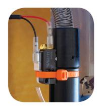
Connect the end terminals of the retractable cable to the two terminals of the micro switch, as shown. The middle terminal is bent down and is not used. There is no polarity to be concerned with.
