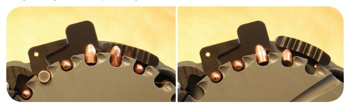
The left image shows the correct ramp position for these 9 mm bullets – the ramp is close up against the collator plate and so the bullets can ride up the ramp and complete their rotation. In the right image, the ramp is positioned much too far out for these bullets, and the bullet tip is missing the ramp and jamming up beneath it.
