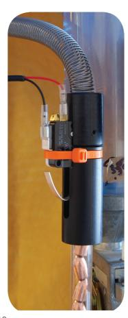
Note the position of the spring's adaptor cap as it attaches to the top of the dropper assembly. Its flat side fits snugly around the micro switch. Note the two wires attached to the outer terminals of the switch.
