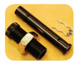
The picture above shows the dismantled dropper lower section. Once the clip is removed, the inner tube can be slid out downwards. Note the three small ball-bearings, which are caliber specific. Always dismantle over a bowl as the small balls will drop out when you remove the inner tube from the threaded body.
