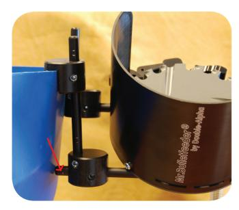
6. Hang the collator back on the rim of your case feeder. Connect the output tube and spring to the top of your dropper and make sure the collator is in the best possible position, allowing the most direct line for the bullets to feed down the output spring. Make sure the spring is not pulling on the dropper. Once you are satisfied with the bullet collator's position, tighten the screws on the inside of the upper pucks to lock the bullet collator in place.
